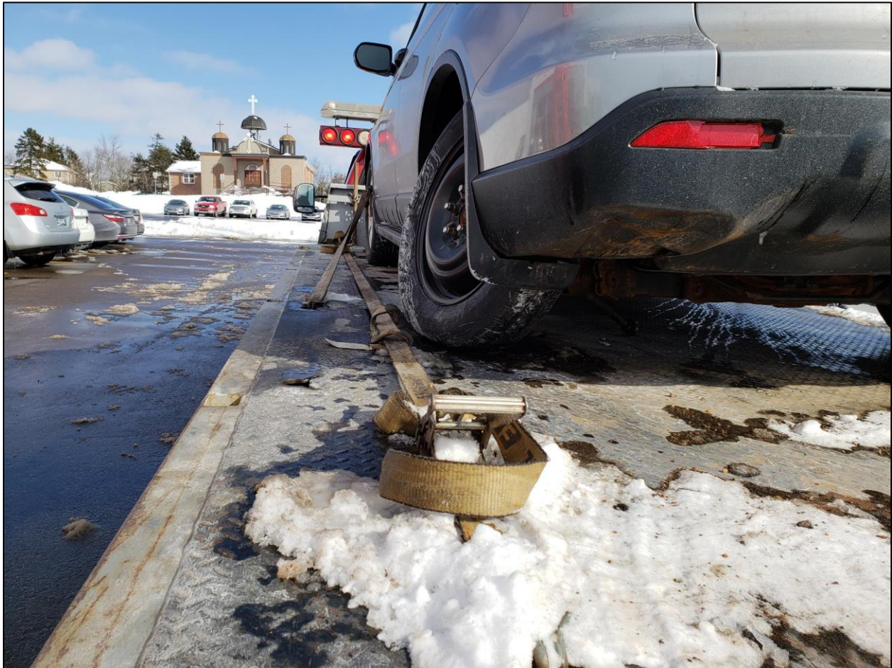
Example of the rear wheel failure that could occur on 2007-2011 Honda CR-V's included in the Honda Safety Recall provided as IR-4 – Attachment 2.
