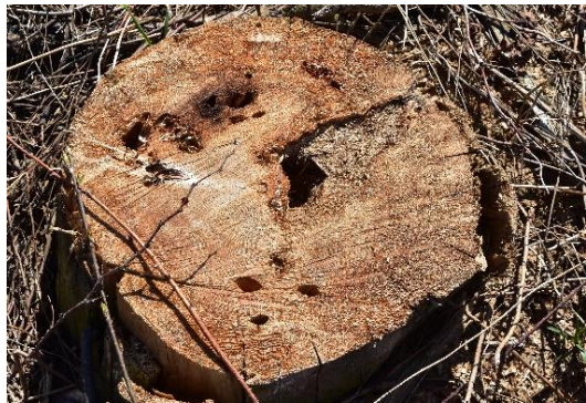
Figure 2-6: Cross section view of decay
