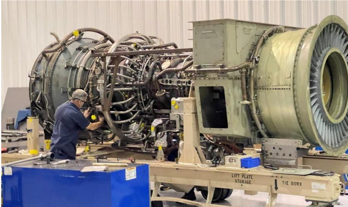
Differentiated Value: PROENERGY combines broad knowledge across the life of the turbine with specialized understanding of aeroderivative engines. Above, a technician helps to perform a complete overhaul of an LM6000 gas turbine.
