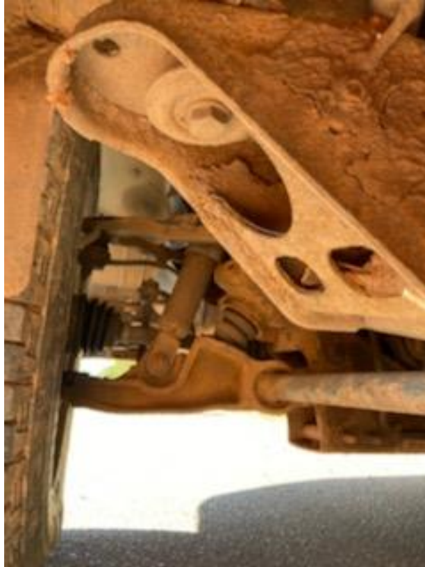
Photo 3 Corrosion of undercarriage on 2012 GMC van
