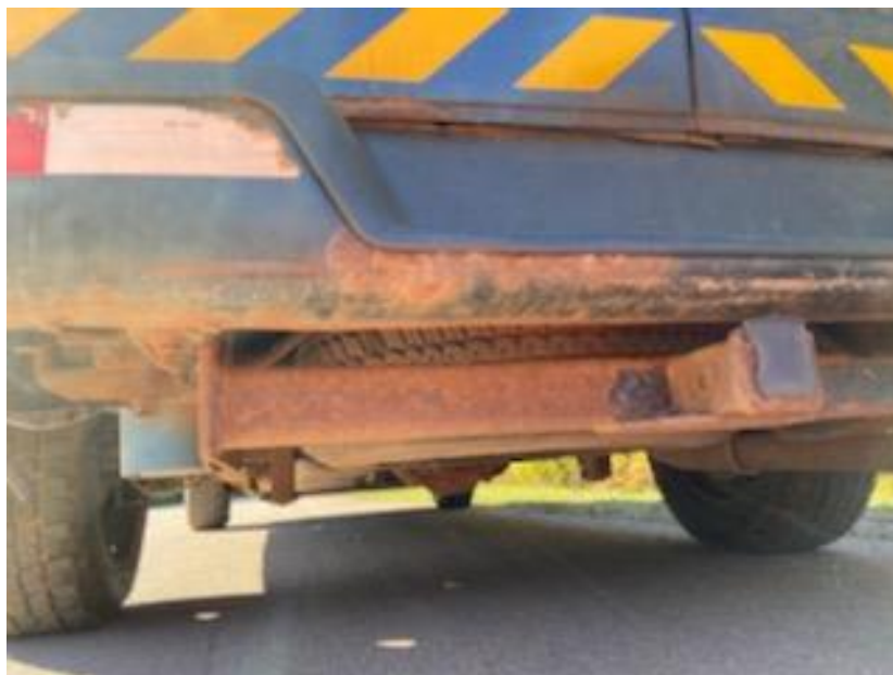
Photo 2 Signs of corrosion on bottom of 2012 GMC cargo van
