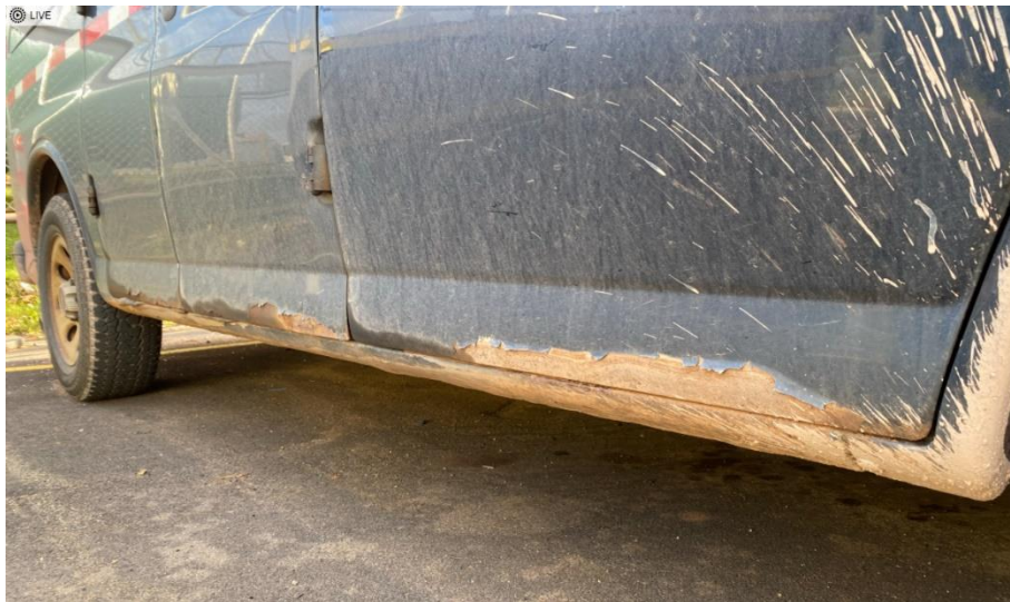
Photo 4 Corrosion along the bottom of door panels on 2012 GMC van
