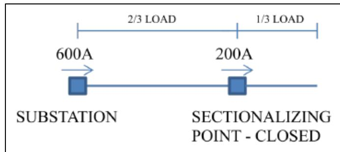
b. After the outage occurs, the sectionalizing point is opened and the substation breaker or recloser is closed. At this point, power is restored to the first 2/3 of customers and the load at the substation is 800 amps (i.e.,  $400 \times 2$ ). After a period of 0.5 to 1.0 hours, the CLPU will have subsided and the normal winter peak load of 400 amps will be present.
